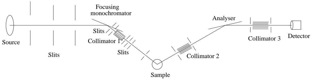
Figure 2: A sketch of the TAS1 instrument at Risø.
